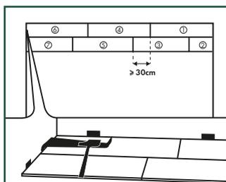
In places where it is too difficult to install the Uniclic® planks with the tapping block (e.g. against the wall), you can pull them together using the pull-bar and a hammer.
