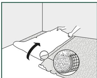
The type of subfloor, its quality and its preparation has a big influence on the final installation result. If the subfloor is not appropriate for the installation of Pergo rigid vinyl then necessary actions should be taken. Contact your Pergo vinyl dealer, who will be more than happy to help you. Be aware that unevenness in the subfloor may leave marks and can create gaps in your Pergo rigid vinyl floor.
