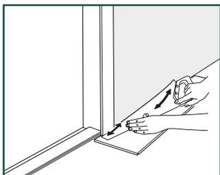
When the new flooring meets a threshold or a doorway, we recommend undercutting the door frames or moldings. To secure the correct cut, turn a plank upside down with the underlay below, and place it on the floor up to the door frame. This ensures that the cut will be made at the correct height. Then place a hand saw flat against the plank and simply cut through the frame. Remove the cut out piece and vacuum away any debris.
