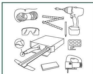
The following standard tools are needed: hammer, saw with blades for plastic (a jig-saw, hand circular saw, hand saw, or cross-cut saw), mouth mask (during sawing), measurer, safety glasses, thin rope, gloves and a pencil. Besides that, you also need the following accessories: Pergo INSTALLATION SET (a pull-bar, spacers and a tapping block suitable for the Uniclic® click system), Pergo Rigid underlay system and suitable maintenance products.
