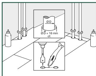
In rows where there is a double pipe, proceed as follows: 1. Measure where the pipe will come through the plank. Don't forget to allow room for the expansion joint. Measure the diameter of the pipe plus 16 mm for the expansion. 2. Drill through the panel where the pipe will come through 3. Extend the hole to the edge of the panel 4. Lay the panel around the pipe
