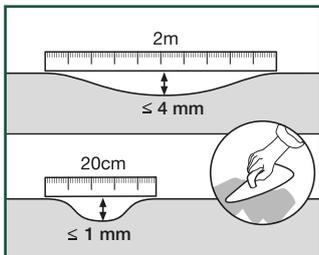
For Pergo rigid vinyl click floors: any unevenness of more than 1mm (0,04inch) over a length of 20cm (7,87inch) must be levelled out. The same applies to unevenness of more than 4mm (0,16inch) over a length of 2m (78,7inch).
