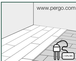
In case of installation on a wooden subfloor, please remove any existing floor covering first. No signs of mold and/or insect infestations should be present. If there is moist in the woodbased subfloor or there is no proper moisture barrier below the woodbased subfloor it has to be removed first. Reason is that the wood will rot after time because the moist is blocked by the new flooring and its underlay.
