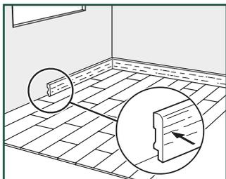
Inspect the final surface of the installed floor. Install PERGO vinyl skirtings against the wall but never attach the skirting to the floor itself. This method allows the floor to expand and/or contract under the skirting-board.
