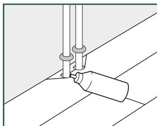
For a perfect finish around pipes, use Pergo pipe covers (floating placement).
