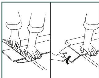
To shorten the length of the plank with a straight cut, you can cut the PERGO rigid vinyl floors with the decor side face up, using a special concave vinyl cutting knife. In order to cut the vinyl plank, draw a straight line along which you will be cutting, and use the knife to make a firm cut in the surface. You never need to completely cut through the vinyl. Then break off the plank using both hands.
