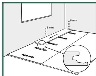
Start with the first plank that will be installed in the corner. Remove the click profile on both the long and the short side of the plank by sawing. For other planks of the first row (not in the corner), remove the click profile on the long side that will be directly next to the wall. Any side of a plank that is directly next to a wall, must have its click profile removed, in order to ensure the required expansion gap.
