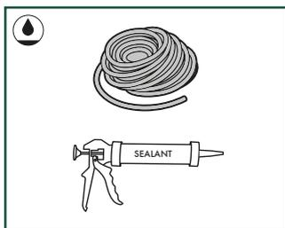
This installation instruction can prevent water infiltration around the perimeter and obstacles of your Pergo rigid flooring. Following these instruction carefully makes the floor fit for use in bathrooms, kitchens, laundry rooms and entrance areas. The water-resistant panels are not suitable for use in damp spaces like pool areas, saunas and rooms with build-in drains like showers. These extra water protection instructions do not cope to national regulations of water protection in wet rooms.
