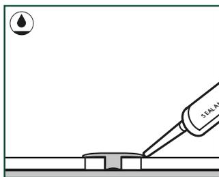
Push the Incizo profile in the base profile and the wet Sealant. Add Sealant where the Incizo touches the floor for a perfect waterseal.
