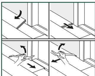
When sawing the panels make sure that the expansion gap under the door is 8mm.
