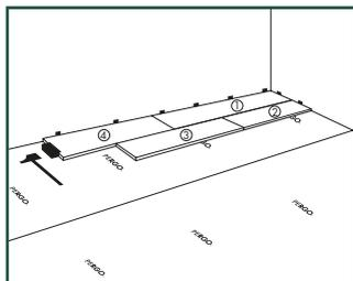
If method A is not possible (at hard to reach places by example), you can use method B (tapping): With Uniclic® you can also join the panels, by tapping the planks into each other, eliminating the need to lift them. This method requires the use of the special Uniclic® tapping block.
