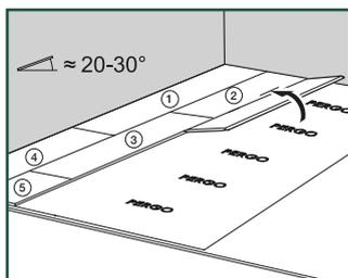
After the installation of each plank and before continuing with the next plank, check each short and long side joint to make sure there are no height differences and no openings.
