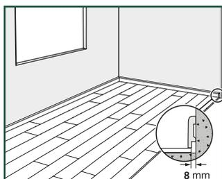
Room temperature varies continuously, so it is vital that the floor is able to expand and contract. For this reason, make sure you leave an expansion gap of 8 mm on all sides of the floor, around pipes, thresholds and under door frames. Expansion gaps can be finished by means of a skirting that is attached to the walls or with an expansion profile. In most cases you don't need an expansion profile between different rooms. However, the use of an expansion profile is mandatory when
