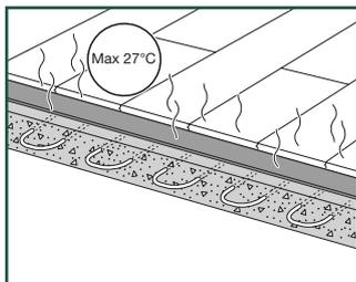
Floor heating systems (water / electricity) which are built-in the screed can be used with Pergo rigid vinyl floors if a constant room & floor temperature of minimum 18°C (64°F) can be guaranteed during acclimatization, installation and 48h after installation.
