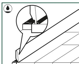
Install the skirting-board with Pergo Multiglu against the wall. When choosing the colour matched skirting or scotia, use the respective hydrostrips to avoid ingress of water and to obtain the look of a cleanly kitted finish. The waterproof paintable skirting can be used without a hydrostrip.
