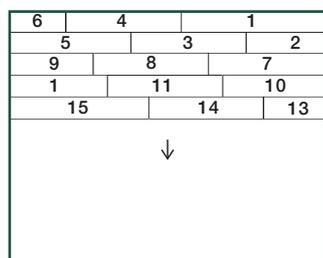
Continue the installation like this - row by row - towards the end of the room. The easiest way to work is to sit on the already installed planks.
