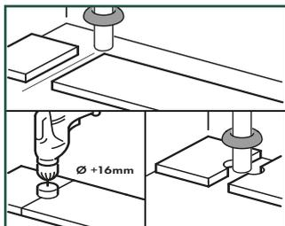
In rows where there is a pipe, make sure the pipe falls exactly in line with the short side of two planks. Take a drill bit with the same diameter as the pipe plus 16mm (0,63inch). Click the planks together on the short side and drill a hole centered on the joint between the two planks. Now you can install the planks.
