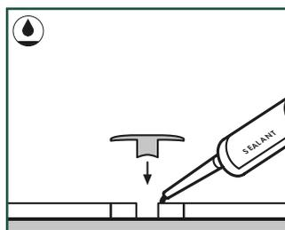
Fix the Incizo base profile to the subfloor with Pergo Multiglu. Apply the flexible Sealant on the PE foam that is in the expansion joint.
