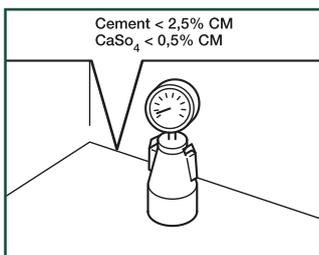
The moisture content of the subfloor must be less than 2,5%CM / 75%RH (cement screed) or less than 0,5%CM / 50%RH (anhydrite screed - subfloor). In the case of floor heating, results must be respectively 1,5%CM / 60%RH and 0,3%CM / 40%RH. Always measure, record and keep your moisture content results.
