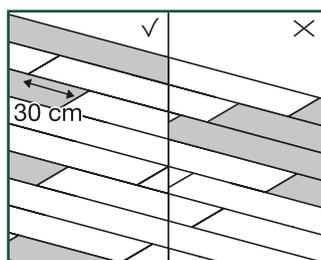
During installation, make sure that you mix the floor panels (and floor boxes) sufficiently so that there are not too many identical, lighter or darker planks next to each other.
